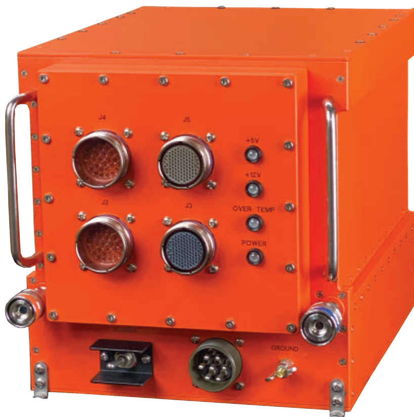
This VITA 48.4 liquid-flow-through ATR box from Elma Electronic has a 6U OpenVPX backplane to accommodate as many as eight computer boards and two VITA 62 plug-in power supplies.
