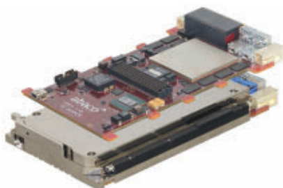
The Abaco Systems VP889 3U VPX field-programmable gate array (FPGA) board offers 100 Gigabit Ethernet for military, aerospace, and commercial embedded computing.
