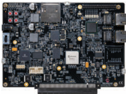
The Microchip PolarFire SoC Icicle kit is a low-cost development platform that enables evaluation of the five-core Linux capable RISC-V microprocessor subsystem, real-time execution, low-power capabilities, and peripherals of the PolarFire SoC FPGA.
