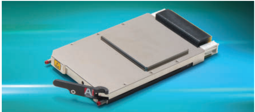
The Aitech C530 3U VPX GPGPU board incorporates the NVIDIA Turing architecture and offers 16 lanes of high-throughput Gen 3 PCI Express and four independent video outputs.
