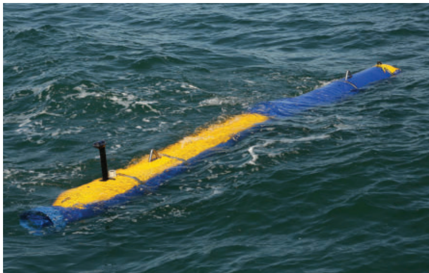
The Knifefish unmanned underwater vehicle from General Dynamics is to be an important component of Navy integrated counter-mine systems.
